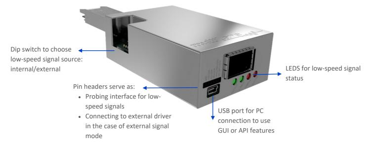
The Nexus Analyzer is used as an 800G verification tool to validate the CMIS/SFF implementation with:
